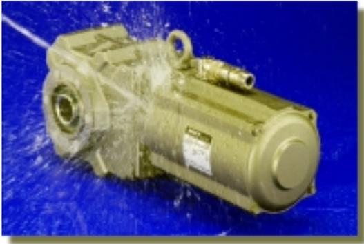
An “aseptic motor” is an asynchronous motor whose basic design dispenses with a fan and cooling ribs. The result is a motor with a completely smooth outer casing which is sealed by a matching non-drive end shield.
