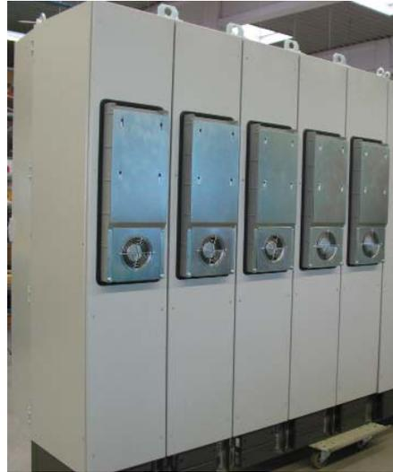
All SPM modules have an IP54 rated heatsink and may be installed with their heat sinks "through panel" mounted. This allows the main cooling to be outside the electronic enclosure, simplifying the design and reducing the thermal stress on the rest of the control system.
