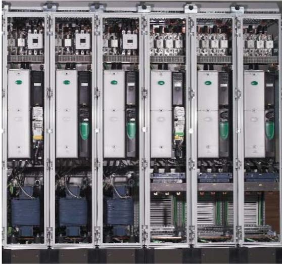
The units that make up the SPM range can be used to implement most types of system. The separation of the power circuit into rectifier and drive stages enables elegant and compact active input configurations to be implemented. For example this 550kW four quadrant test rig system consists of 6 identical drive modules in a 2.4m cubicle suite.
