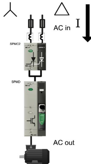
Multi-pulse rectifiers can be configured (12, 18 and 24 etc.), to minimise input harmonics and help to meet local supply authority regulations.
